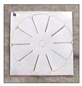
I've made a template from 1mm (0.040") stainless steel and I simply press this against the prepared reed valve material and scribe around the edges with a sharp modeling knife. Don't forget to also scribe the hole in the middle!
